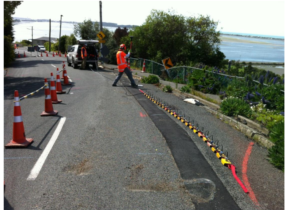
Figure 5 MASW field operations.
